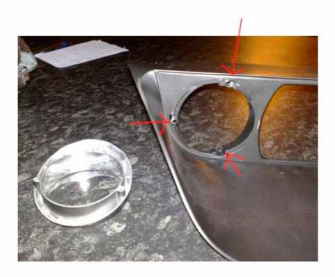
**5.** Take the ring and work out where you want the wire to be hidden or run. I mounted mine by drilling a hole directly through the bottom of the insert then feeding the wires back between the insert and headlight.
