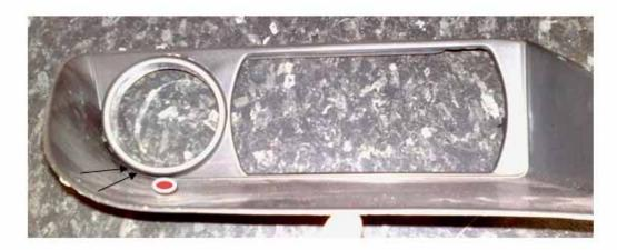
**6.** Next is to mount the Angel Eye to the projector ring. To do this I put a few very small blobs of Araldite on the projector ring and stickytaped the Angel Eye in place till it dried. Be sure to make sure the wires are facing in line with the drilled hole so you can feed them out through. One note when using araldite and sticky tape, try not to glob the araldite under the eyes as it may run onto the stickytape and then onto the outer side of the projector ring.
