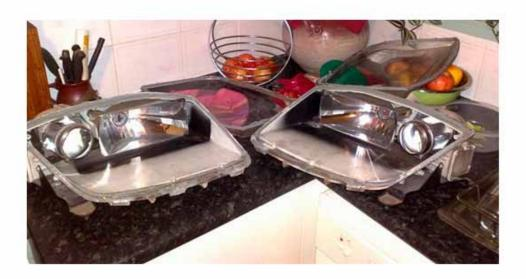
**3.** Next step is to remove the headlight insert, to do this there are 2 small screws at the front of the insert. Dig the sealant out from where the screws are, then undo them and remove insert.
