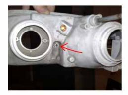
Then sit the insert back in, making sure the two locator pins on each side line up, then screw back in place with the front mounting screws. Don't force it in if it doesn't want to go in, as by the time you finish this things may have cooled down considerably and contracted. Take your time, you will get it back in place.
