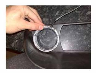
7. Once dry enough to move around, feed wire through the hole and screw the projector ring back in place. Now would be a good time to test the eyes out with your black inset panel. Just connect the pos / neg to a car battery or a 12V.
