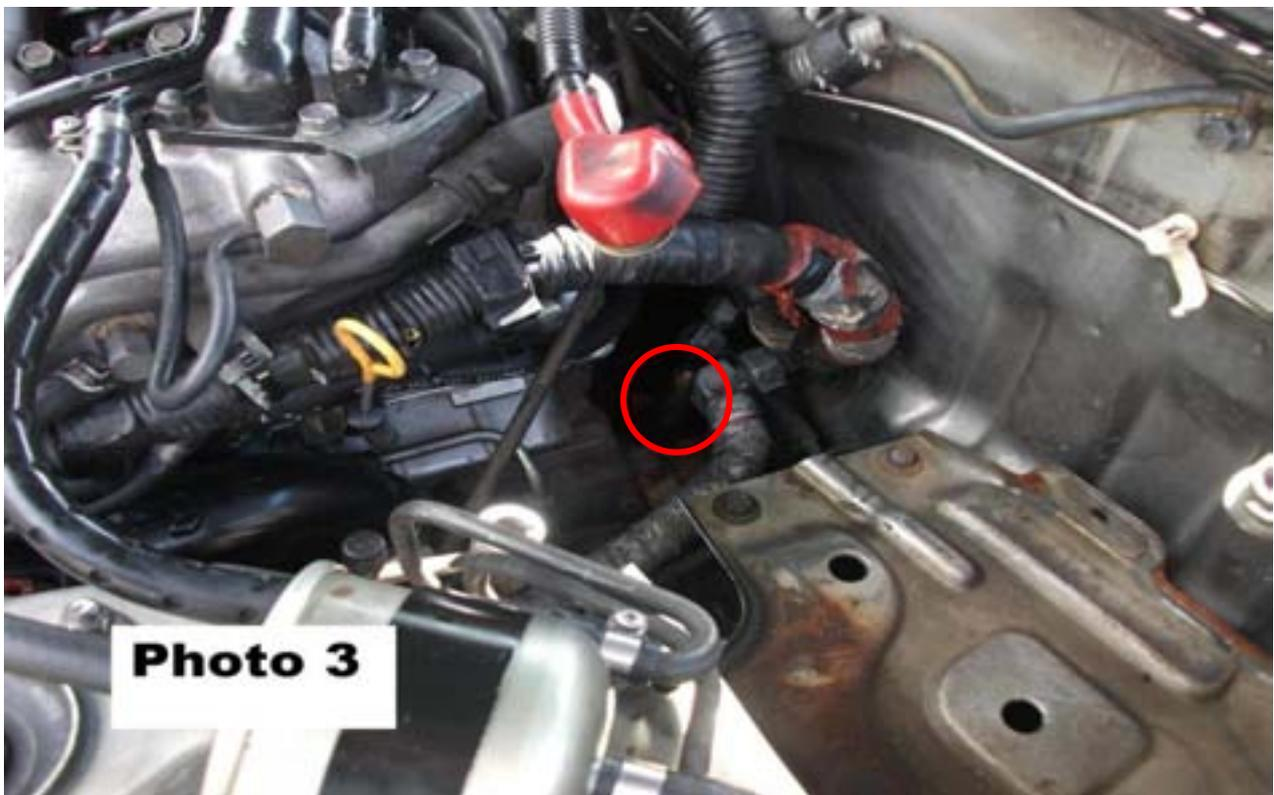
The O2 sensors are tucked back behind the engine on the exhaust manifolds, one on each side of the engine. The passenger side one is easier to see and reach with the battery removed (Photo 3). The driver's side one can be seen by looking down passed the brake booster (Photo 4).
